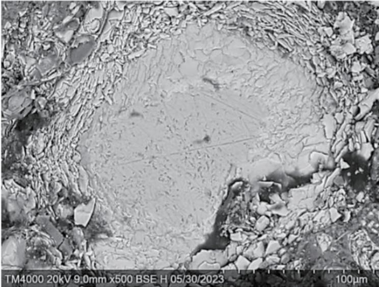
Figure 4 – SEM image of fragment 2 Figure 1. Calcium-containing core (dark gray) and multilayer «shell» containing strontium.
